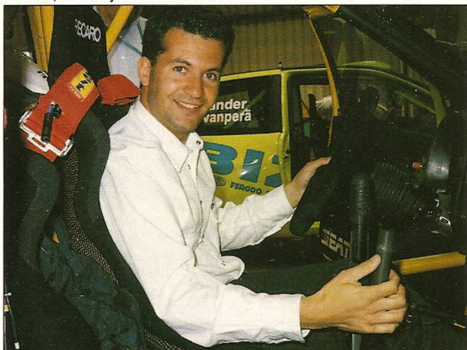
1997 Seat works driver Oriol Gomez demonstrates the Evo 2 Ibiza Kit Car's unusual, vertically mounted handbrake.
